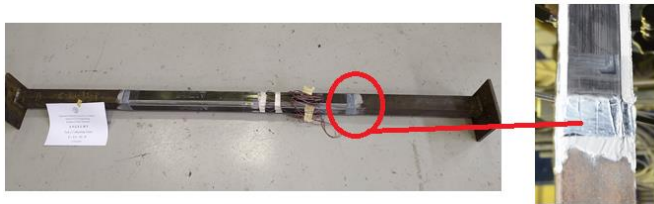
Figure 1 Hybrid specimen with confined CFRP ends
