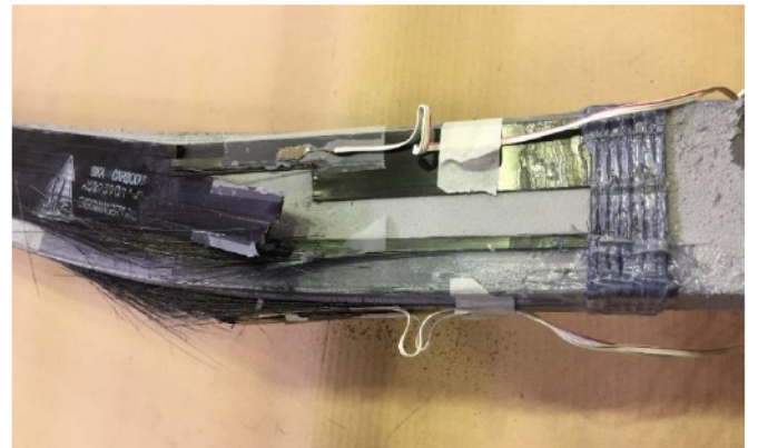
Figure 7 Types of failure for CFRP. Debonding from steel for compression and fracture of fibers for tension
